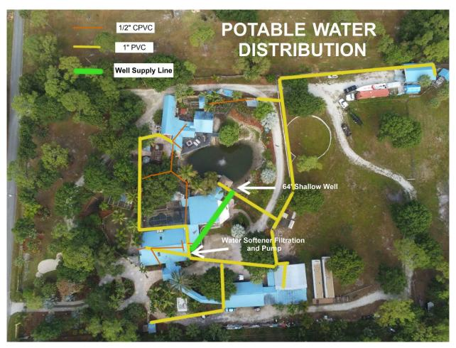
Figure 44-Potable Water Distribution
