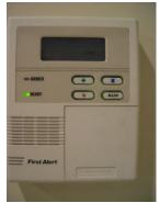
Figure 88-First Alert Control Panel
