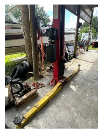
Figure 102-9,000 LB Hydraulic lift
