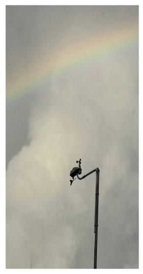
A DAVIS Vantage Vue weather station is mounted atop a 40' mast on the Primary dwelling. It is solar powered and feeds a signal via Bluetooth to a panel mounted
